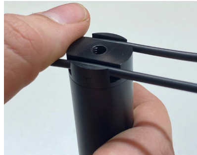
Fig 8.1 Align slots in the luminaire head.
