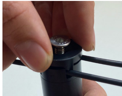
Fig 8.2 Fit the cap
