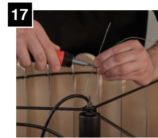
17 Tighten both screw of strain relief and adjust aircraft cable length as needed. Cut loose aircraft cable if necessary.
