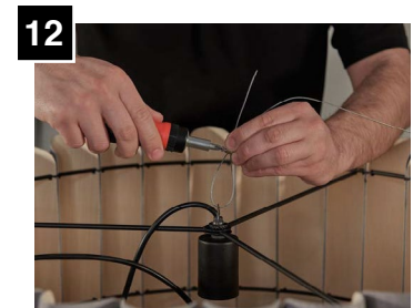
Tighten both screw of strain relief and adjust aircraft cable length as needed. Cut loose aircraft cable if necessary.
