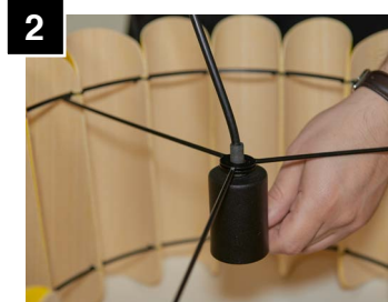
2 Pull cord until socket bottoms out. Socket assembly with extension rod ensure nut is below ring before proceeding to step 3 (lock washer and nut/balancer)
