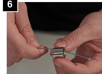
6 Completely feed aircraft cable through coupler, until stop is reached.
