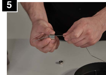
5 Twist off end cap from cable coupler and feed aircraft cable.
