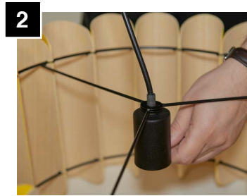
2 Pull cord until socket bottoms out.
