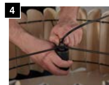
4 Firmly tighten socket to shade ring.
