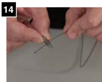
14 Pass aircraft cable through one hole of strain relief.
