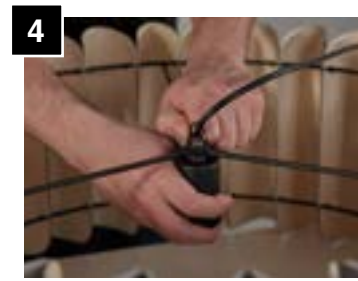
4 Firmly tighten socket to shade ring.
