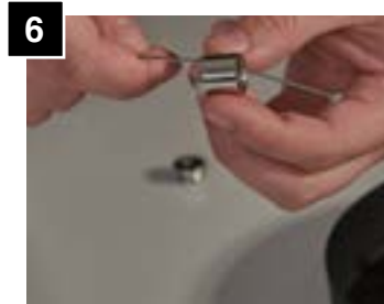
6 Completely feed aircraft cable through coupler, until stop is reached.
