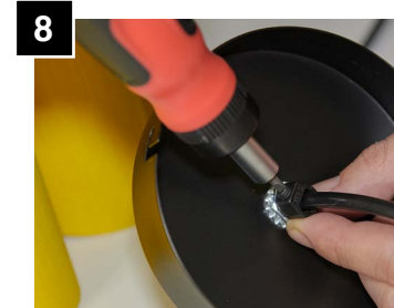
8 Slide down until it bottoms out and tighten set screw.
