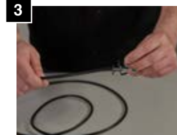
Feed lock washer and nut/balancer through cord.
