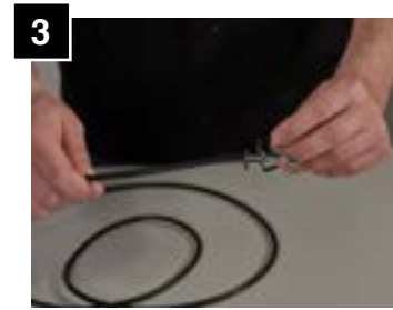
Feed lock washer and nut/balancer through cord.
