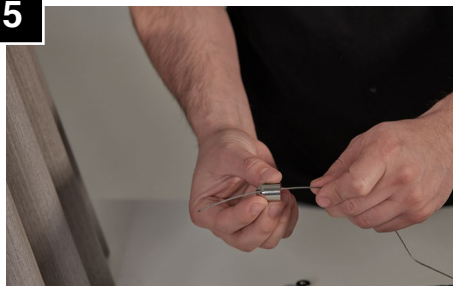
Twist off end cap from cable coupler and feed aircraft cable.
