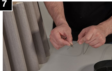
Pass aircraft cable through one hole of strain relief.
