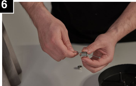
Completely feed aircraft cable through coupler, until stop is reached.
